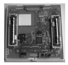
Ensure that the batteries are inserted correctly, paying careful attention to the polarity markings on the battery and next to the battery holders. After inserting the batteries, refit the ST620 case and retighten the securing screw.
