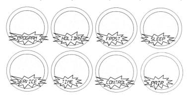
You can scroll through the menus in either direction (forwards or backwards) depending on the direction you move your finger around the Touch Ring. The menus are displayed in the order shown in the picture above.
