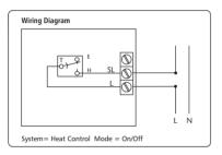
There are only two electrical connections required to the ST320, and these connections should be made to the terminal block inside the thermostat. No Earth connection is required for the correct and safe operation of the ST320, but a parking terminal is provided to connect an Earth wire if one is present. These connections are shown in the drawing and table below:
