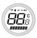
The display consists of a combination of symbols and alphanumeric displays. The top row is a set of status symbols, the centre row is used to indicate temperature (in Celsius), and the bottom row is an alphanumeric display for menu and status messages.
