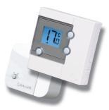
The Receiver is used for wiring connections and heat on/off control. The Control Centre provides the user interface and temperature sensing / control. The two units are linked together by a Radio Frequency (RF) signal.
